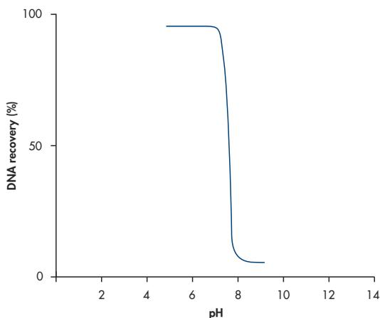
**Figure 1** pH dependence of DNA adsorption to silica. 1 µg of a 2.9 kb fragment was adsorbed at different pH values and eluted with 10 mM Tris-Cl, pH 8.5. The graph shows the percentage of DNA recovery, reflecting the relative adsorption efficiency, versus the pH of adsorption.
