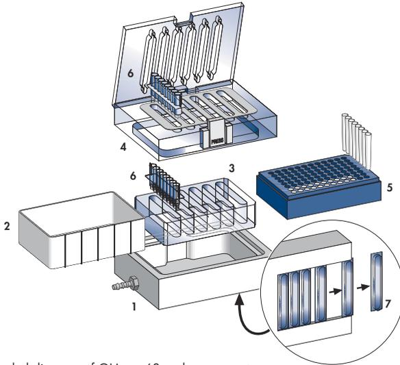
**Figure 2** Exploded diagram of QIAvac 6S and components
